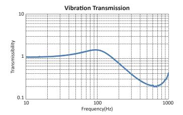
Testing condition Sample: □ 5mm, t=3mm
