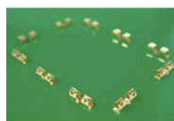
Shield-can clips reflow soldered onto PCB
