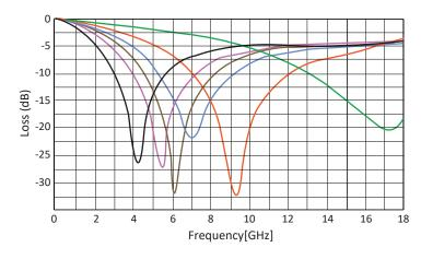
Performance comparison of NSSR material in different thicknesses targeting 15GHz
