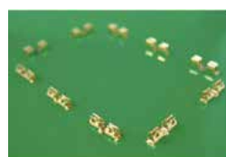
Shield-can clips reflow soldered onto PCB
